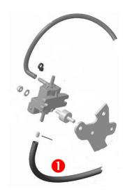
To fit the impulse nozzle • (part RTX 956 305) into the pressure hose is optional. The direction of the impulse nozzle inside the pressure hose is free.
